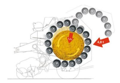
MPS II – with pressures up to 1.4 tons (1.3 tonnes) for a highly compacted bale core and a powerful 20% increase on MPS I in closing pressure to 5.3 tons (4.8 tonnes) for bale compaction, the ROLLANT delivers perfectly compacted bales.
