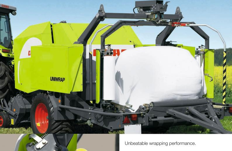
CLAAS has designed the UNIWRAP with dual 750-mm wrapping arms that allow a bale to be stretch-wrapped with six layers of stretch film and a 52% overlap in just 25 or 35 seconds (depending on model), finishing its job before the next bale is ready. The ROLLANT can continue at full speed even when wrapping.
