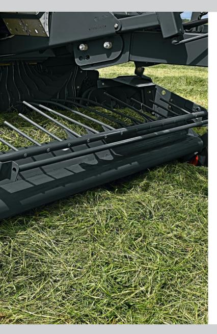
With its 6.9 ft (2.1 m) working width and 130 rpm in the 455 or 125 rpm in the 300 range, the pick-up can take in even the widest windrows thoroughly without damaging the crop. Large caster guide wheels keep it securely on track. The short crop guard guides the flow of forage safely to the rotor, even in small and irregular windrows. The pick-up follows every ground contour and protects the grass cover, even at high operating speeds and when turning.
